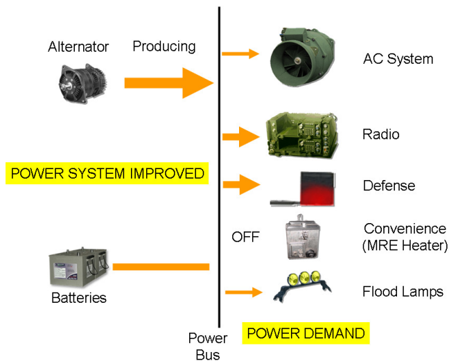
Figure 3 – Power System Improved Through Power Management
