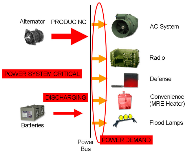
Figure 2 – Power System CRITICAL
