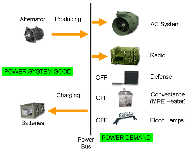
Figure 1 – Power System GOOD
